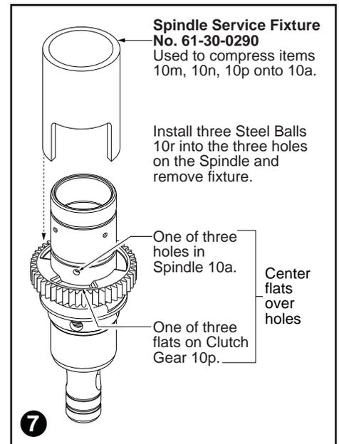
**Assembly of external Spindle components:**
