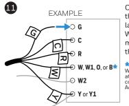
Connect the wires from the "Equipment" labelled side of the C Wire Adapter to the matching terminals on the control board.
