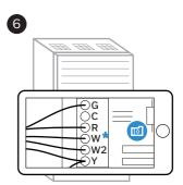
Take a picture of the wires on the control board.
