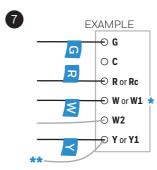
Use the provided stickers to label the following connected wires:
