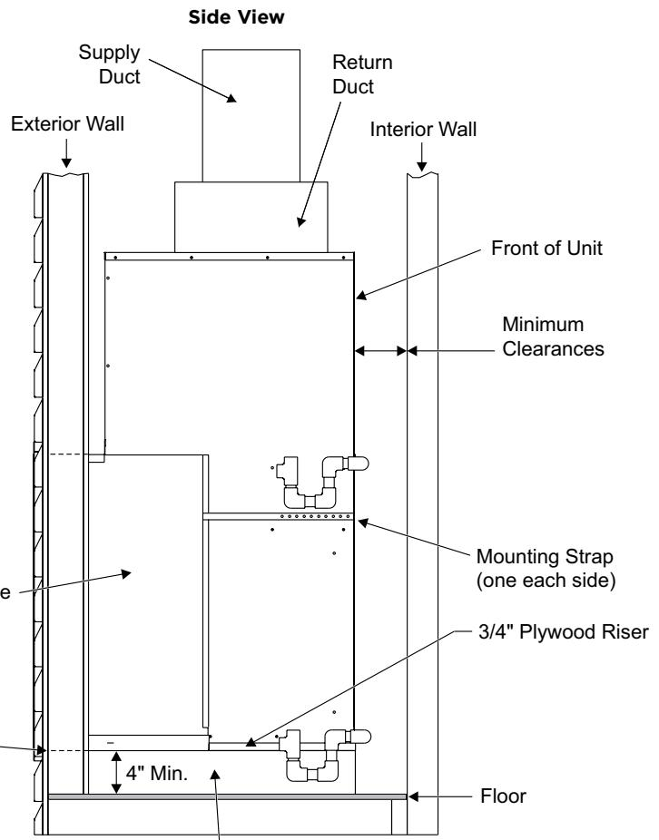
Platform (field supplied) - Unit must be supported by platform, which must be level with sill plate of opening in exterior wall.
