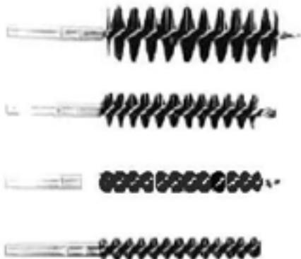
Condenser tube and heat exchanger brushes are available in two bristle materials: stainless steel and brass. Bristle sizes are graduated from 0.006" on small diameter brushes to 0.012" on larger sizes to provide consistent cleaning power. There are not OD threads on 3/8" brushes. Shank length is 2". Adapters are also available to accommodate other standard thread sizes.
