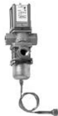
Maximum permissible bellows pressure for R-12 is 230 psig (1586 kPa) and for R-22 is 320 psig (2206 kPa)
