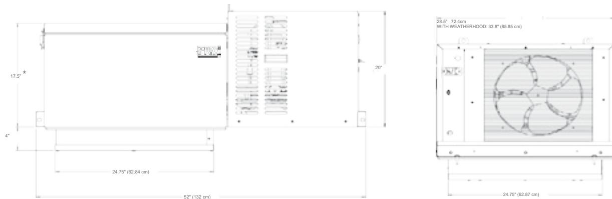
**25"X25" PANEL OPENING REQUIRED FOR EVAPORATOR SECTION OF "P2" CABINET SIZES.**
