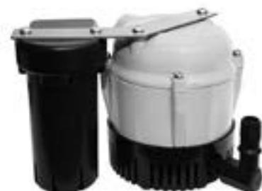
**2-ABS:** 1/2 gallon tank, 1/4" MNPT discharge, with On Level - 3" Off Level - 2", 11.8' shut-off.
