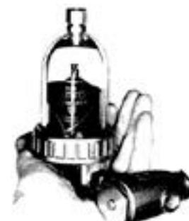
When condensate level rises, float lifts, allowing air under pressure to flow through the hollow stem into the auto-drain where a diaphragm distends with increasing pressure and opens a large scavenger-action dumping valve. Float drops and the control unit waits for the next accumulation.
