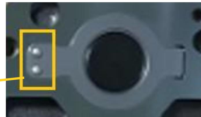
Suction reed riveted on valve plate
